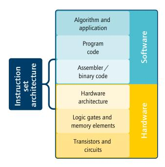
Figure 1: Layers of a computer system (source: own presentation)
