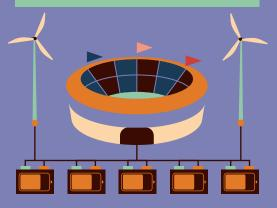
The purpose of this energy storage system is to supply the stadium with sufficient electricity from renewable sources, such as solar or wind energy. If the weather changes and the wind and sun stop playing along or if demand spikes during a game, the e-battery steps in and balances the power supply.
